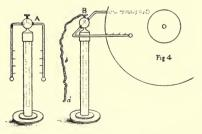
"A represents the machine with the arms shut laterally as placed in case; B, the machine as placed in its relative position on one side of the glass plate, a.b. a chain to communicate with the prime conductor, placed in any convenient situation.
